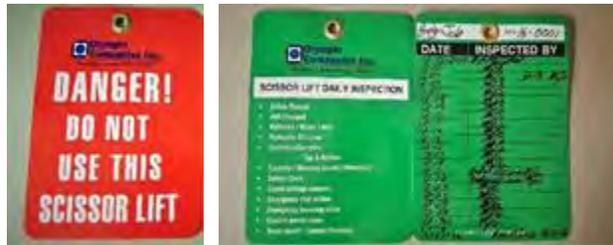
The "operator of the lift" is responsible to inspect the aerial lift prior the start of each work shift. This procedure needs to be completed to verify that our work place, and the equipment we use, is in safe working order.
